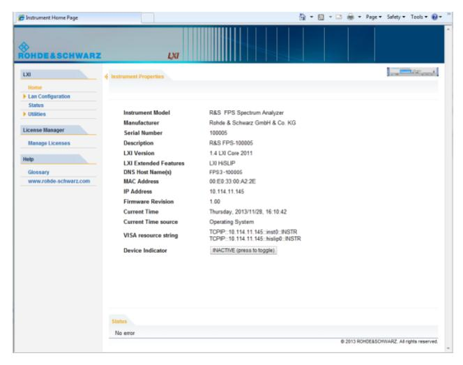
The instrument home page displays the device information required by the LXI standard including the VISA resource string in read-only format.
