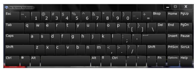
The on-screen keyboard display can be switched on and off as desired using the "On-Screen Keyboard" function key beneath the screen.
