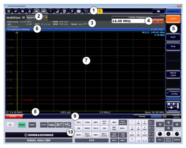
Fig. 6-1: Graphical user interface elements in the R&S FPS's soft front panel
