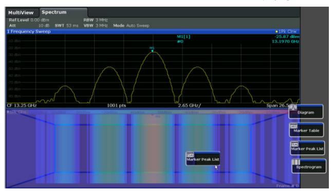
Fig. 6-4: Moving a window in SmartGrid mode
