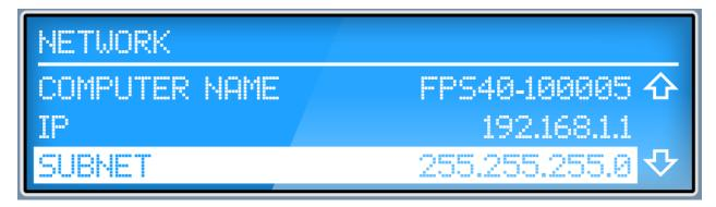
The R&S FPS is equipped with a miniature display on the front panel that provides basic information and allows for very basic instrument configuration (such as changing the IP address). For details see chapter 4, "Miniature Display", on page 37.
